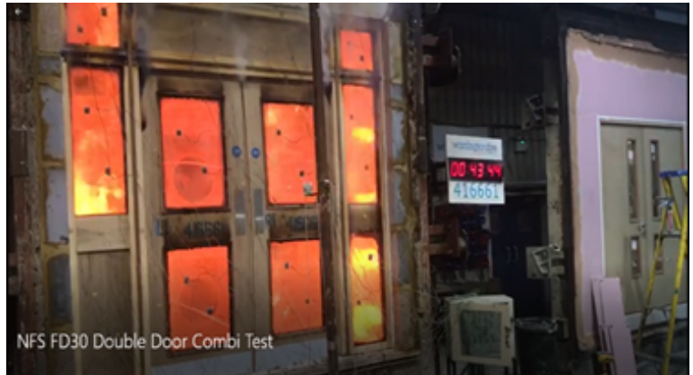
FD30 burn test carried out at Warringtonfire UKAS laboratory. Our tested configuration is far more onerous than tested by our competitors (as shown to the right on the unburned double doors) and pushes the envelope to offer larger glazed and solid options. This sample achieved 43mins 50 secs far exceeding the 30min standard.
