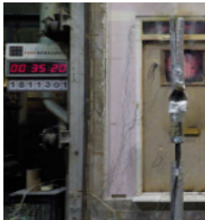
FD30 burn test carried out at Cambridge Fire Research UKAS laboratory. Our tested configuration covers our PAS24 Enhanced Security doorsets with fanlights from both sides.
